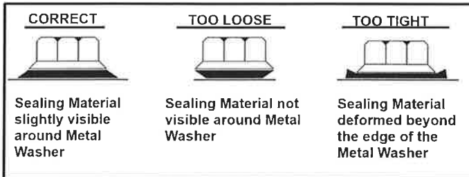
THIS CHART SHOWS PROPER FASTENER SEATING PRACTICE
