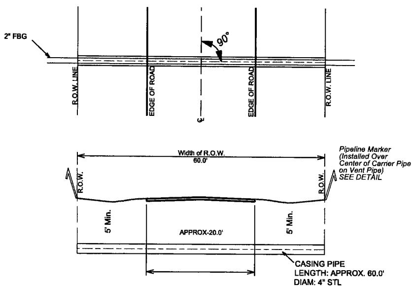
Note: Vent Pipe to be installed on each end of casing. Minimum of 2' above natural ground.
