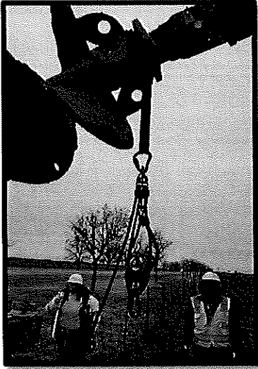
Figure 2. The rope/carabiner will be setup with the rescue system on the anchor point and above the braking system. Rope is positioned above hoist.
